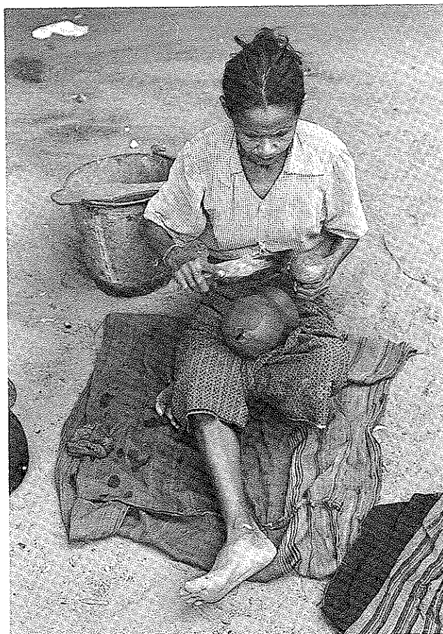
Plate 1: Woman in the modern village of Ban Kham Oo, shaping a globular vessel with a paddle and anvil. (Photograph: Courtesy of Joyce White, Asian Section, The University Museum.)
