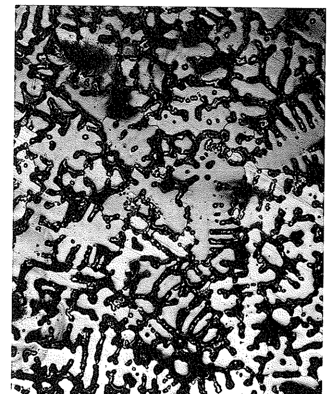
Figure 15.10 Bracelet/anklet BCES 708/1594, a low-tin bronze (5.6%), was left in the as-cast condition. \times 100 .
